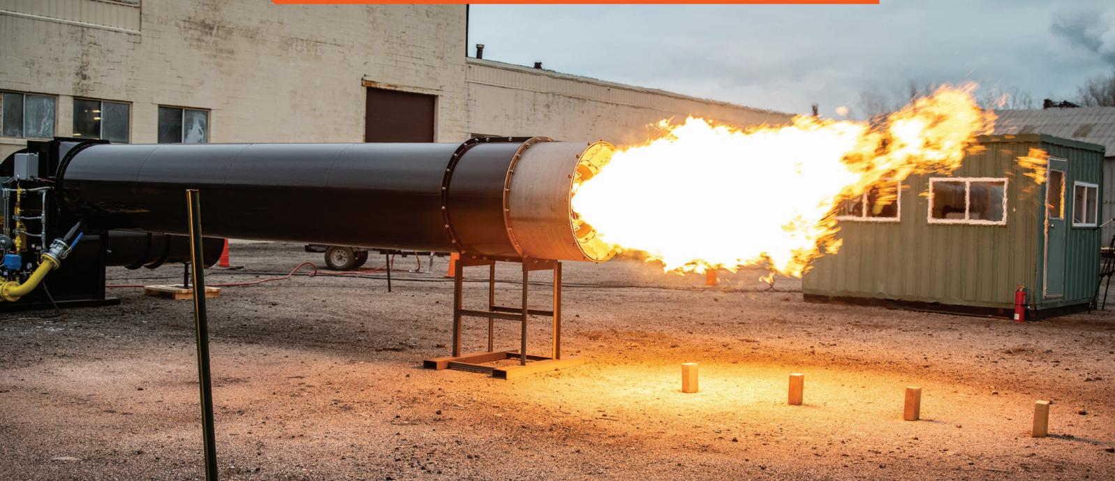
This HADES-125 burner from Detroit Stoker is being factory test fired on fuel oil.
