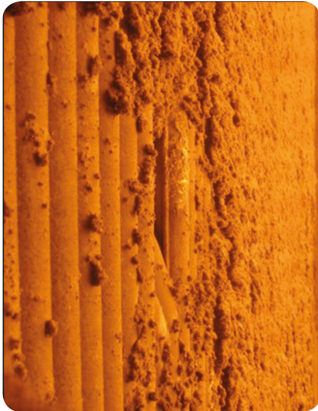
Figure 2a and 2b: Biomass boiler slag and clinker formation.
