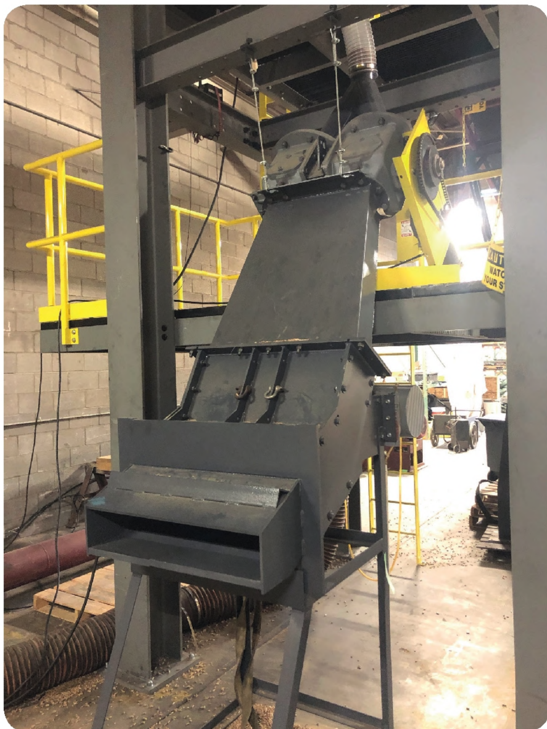
Figure 11: Pellet metering testing in R&D test facility.
